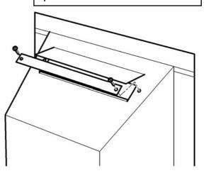
Figure 13. Flue restrictor
