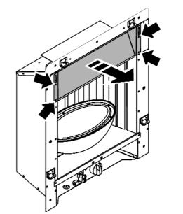
Figure 31. Spillage plate removal
