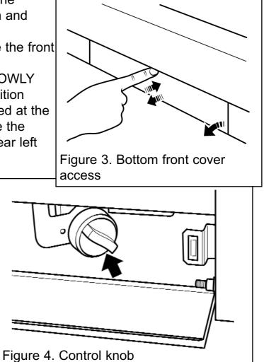
partially depress the knob and turn to "LOW". The pilot should then light the main burner at its low setting. There may be a delay of up to four seconds between the pilot lighting and ignition of the gas at the main burner. This is normal and is due to the time required to fill the main burner compartment with sufficient gas for ignition.
