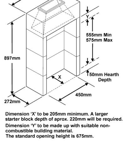
Figure 7. Precast or clay flue block system dimensions
